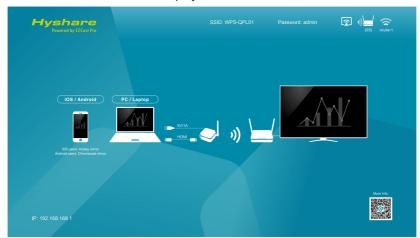
4.1.3 SSID and Password: The user may see the required information for connection at the upper middle of the standby screen.
